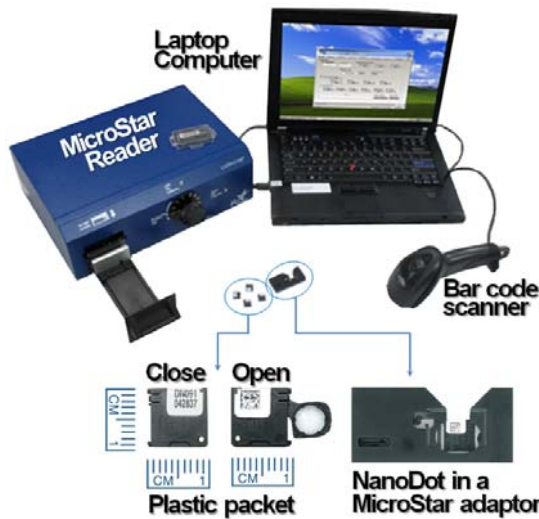
Fig. 1. InLight™ OSL system. The MicroStar reader is a compact, lightweight, portable reader. OSLDs are plastic discs infused with crystals of Al 2 O 3 :C and little build-up in device itself.
