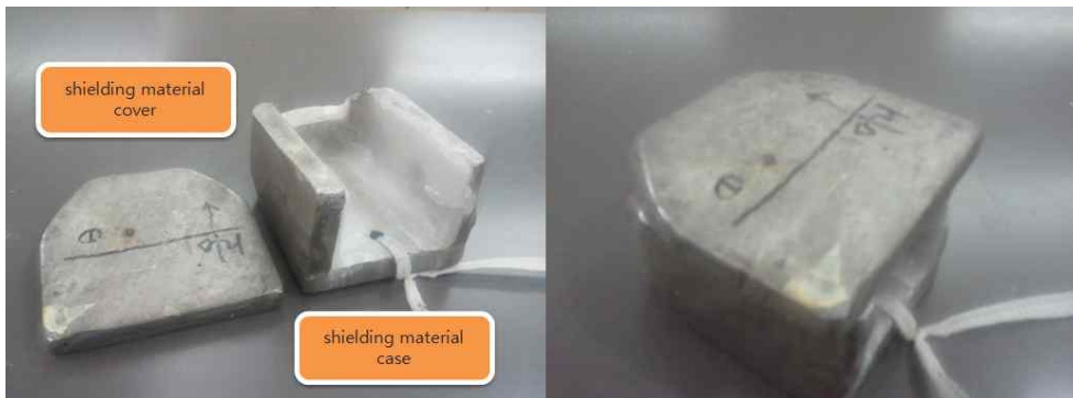
Fig. 1. Gonad shielding from scattered photon with lead shielding material. The shielding material consists of case with 3 layers and a cover (left). The cover is placed on the case in order to protect gonad (right).
