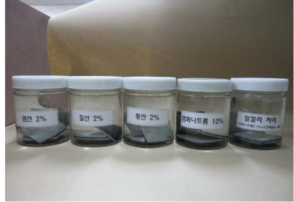
Figure 12. Chemical resistance test
