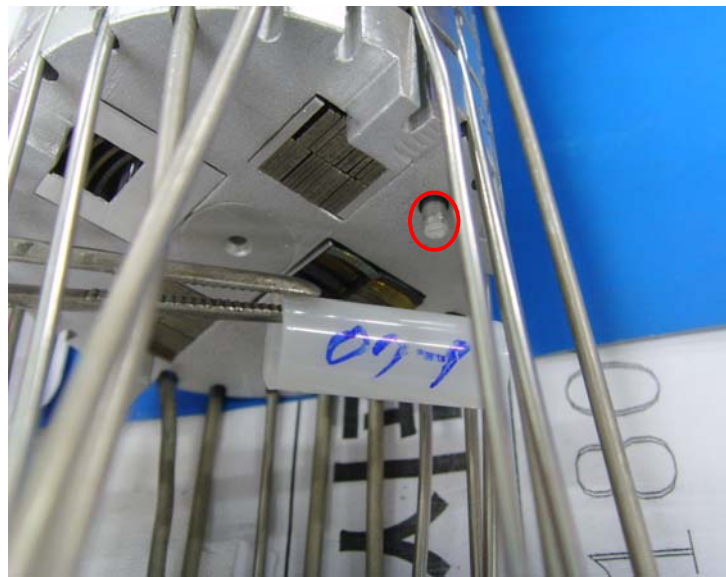
Fig. 3. The mounted F/M sample to perform the experiments in HANARO research. (red circle in figure)
