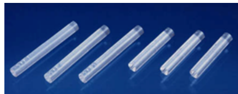
Fig. 3. Glass dosimeter used for patient dose measurement.
