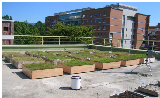
Fig. 1. Shallow-extensive green roof experiment view treated with different soil thickness and soil mixture at Konkuk Univ. in Chungju.
