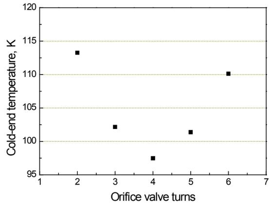
(a) no-load temperature as valve opening
