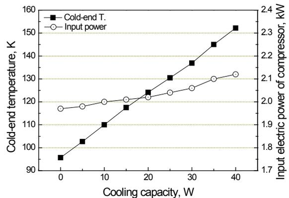
(c) cooling capacity and compressor input power
