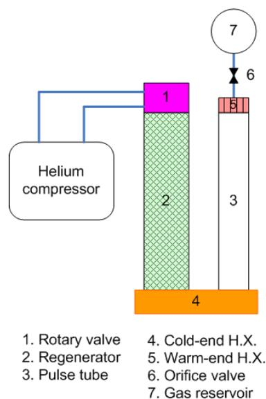
Fig. 1. Schematic diagram of single stage orifice pulse tube refrigerator.
