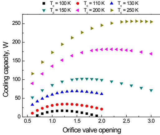
Fig. 3. Cooling capacity variation as orifice valve opening and cold-end temperature.
