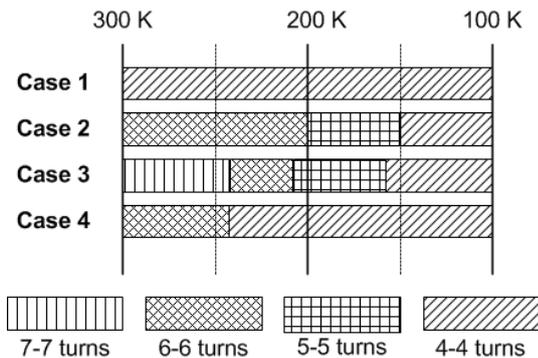
Fig. 7. Scenario of orifice valve control during initial cooldown process.
