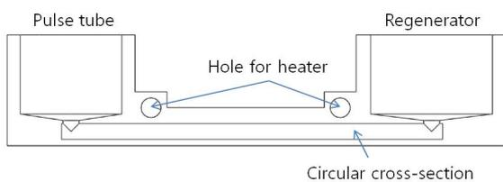
Fig. 5. Cross-section view of cold-end.
