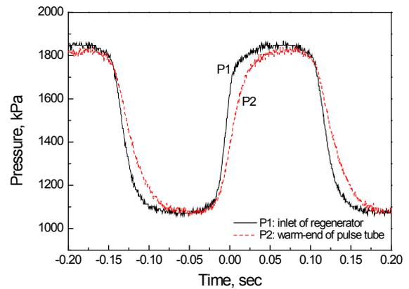
(b) measurement of pressure waveform
