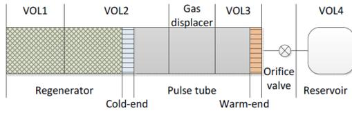
Fig. 2. Schematic diagram of isothermal model.
