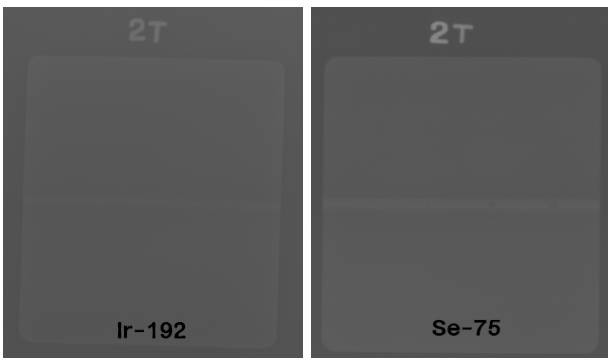
Fig. 7. Images of plate object with hole defects of diameter 0.5, 1, 2, 3 mm and 2 mm thickness ( 192 Ir : left, 75 Se : right).
