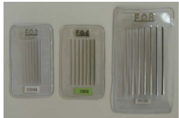
Fig. 11. Photograph of wire-type image quality indicator (IQIs).
