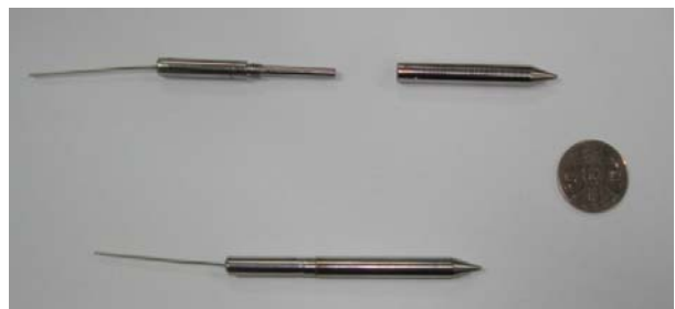
Fig. 2. Ionization chamber to measure the gamma-ray profile of spent fuel.
