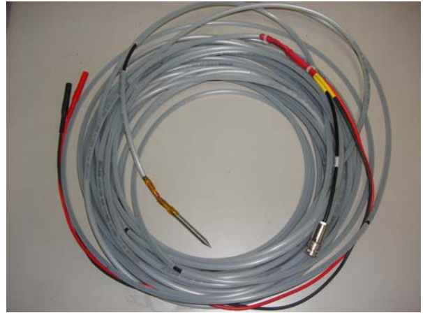
Fig. 6. Assembled Gamma probe to measure the gamma-ray from spent fuel.
