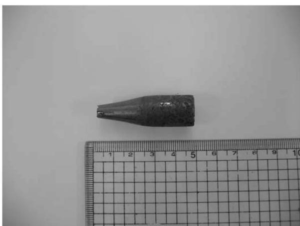
Fig. 1. CZT crystal grown with the low pressure Bridgman method.
