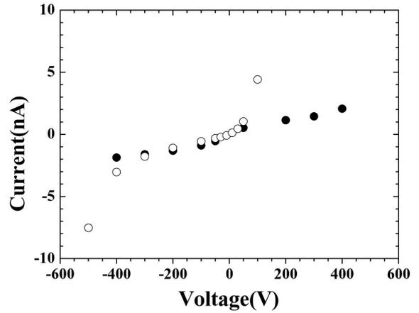
Fig. 4. I-V curve of CZT detector, where the crystal was grown with high pressure Bridgman method. The closed circles are the leakage current of the CZT resistive detector, and the open circles are the leakage current of the CZT Schottky detector.
