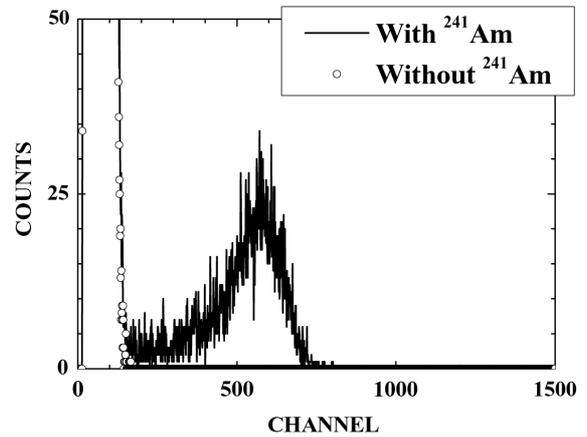
Fig. 5. 5.4 MeV  $\alpha$ -energy spectrum measured with CZT Schottky detector. The crystal was grown with the low pressure Bridgman method.
