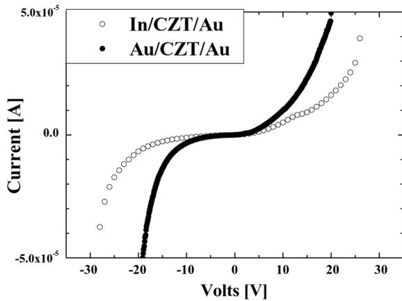
Fig. 3. I-V curve of CZT detector, where the crystal was grown with the low pressure Bridgman method.
