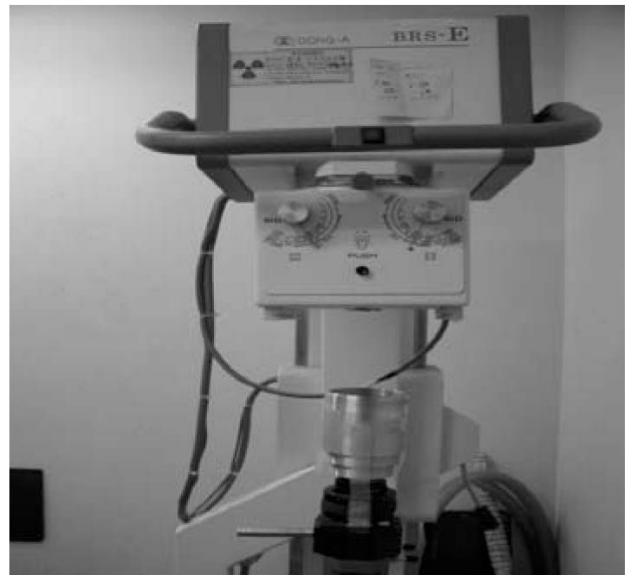
Fig. 9. The CCD image sensor with an optical lens set.
