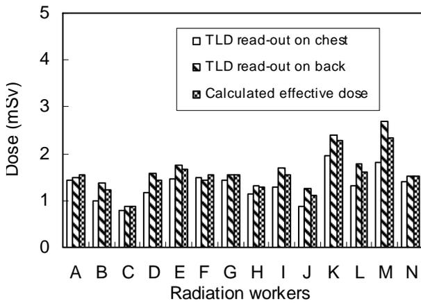
Fig. 5. TLD readouts for the plugging and nozzle dam removal of steam generator at Yonggwang NPP No. 1.
