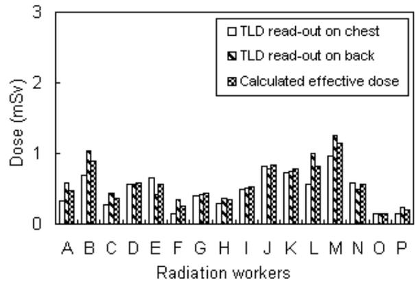
Fig. 3. TLD readouts for the penetration test of a reactor head at Kori NPP No. 1.
