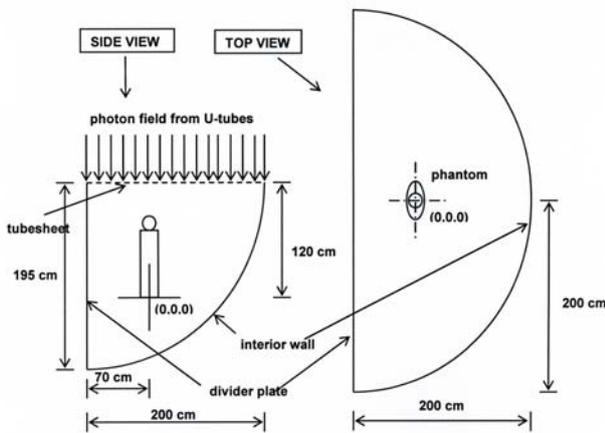
Fig. 1. Source geometry of steam generator.
