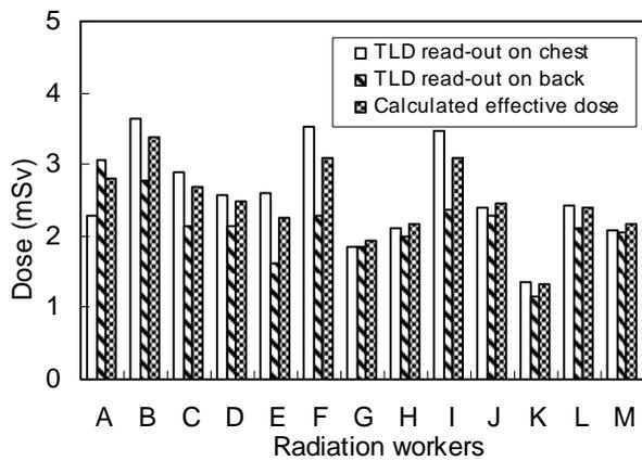
Fig. 6. TLD readouts for the ultrasonic test of feeder pipe at Wolsong NPP No. 1.
