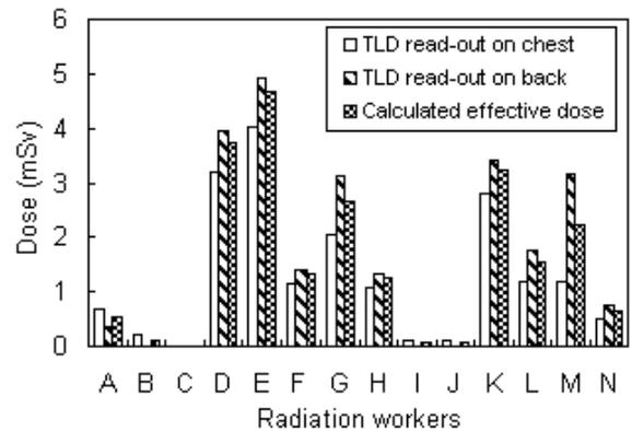
Fig. 2. TLD readouts for the installation of a steam generator nozzle dam at Kori NPP No. 1.
