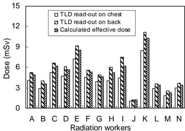
Fig. 4. TLD readouts for the installation of a steam generator nozzle dam at Yonggwang NPP No. 1.
