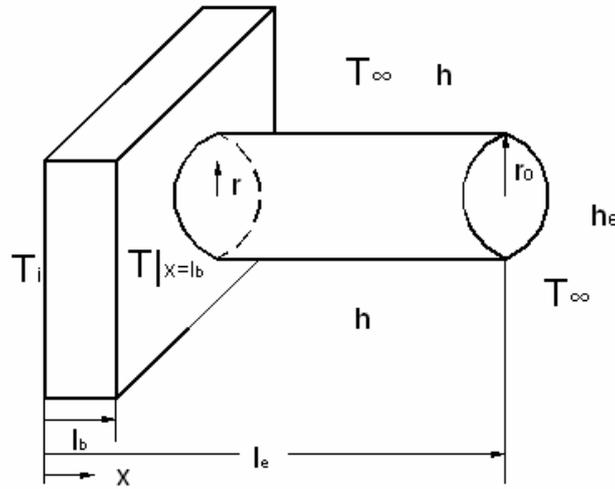
FIGURE 1. Schematic diagram of a pin fin
