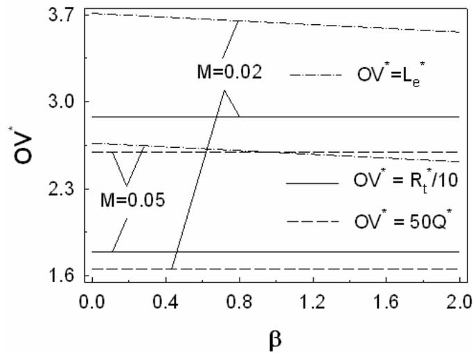
FIGURE 5. Optimum values versus convection characteristic numbers ratio ( $L_b=0.1, R_o=0.15$ )
