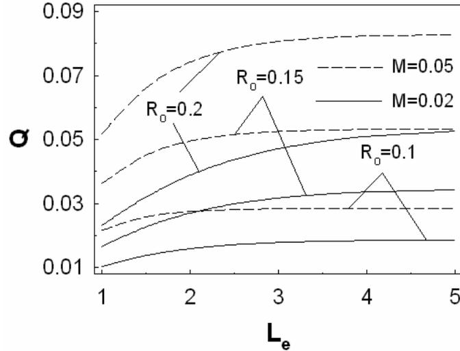
FIGURE 2. Heat loss versus the fin length ( $L_b=0.1$ ,  $\beta=1$ )
