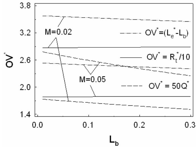
FIGURE 3. Optimum values versus the fin base thickness ( $R_o=0.15$ ,  $\beta=1$ )
