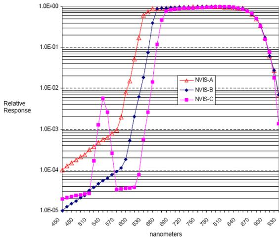
[Figure 2] Relative spectral response characteristics of Classes A, B, and C NVIS
