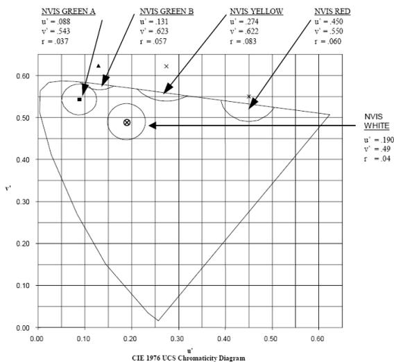
[Figure 4] NVIS lighting color limits
