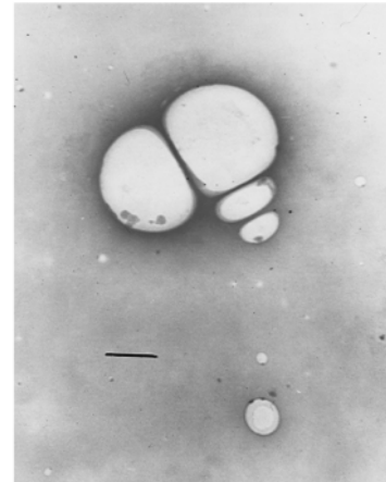
Figure 3. TEM images of ULVs obtained from octasubstituted cyclophosphazene without DHPP (bar represents 200 nm).
