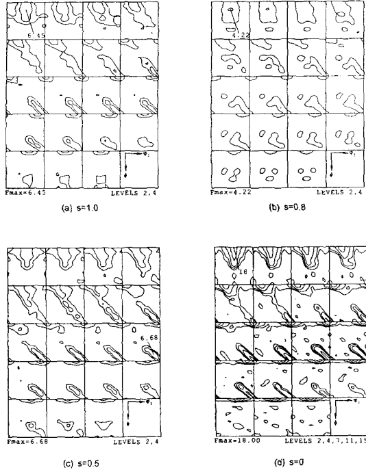
Fig. 10 Cold rolling texture of the ferrite stainless steel after 40 % thickness reduction (32)
