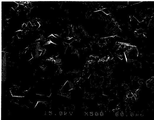
Figure 4. SEM photograph for cobalt oxide at the mixer temperature of 350 °C (reaction temperature and pressure: 400 °C and 340 bar).
