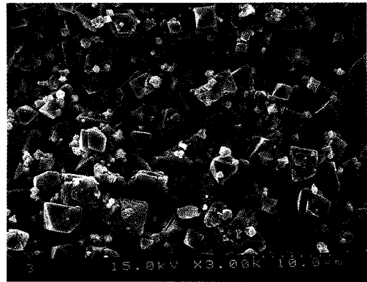
Figure 6. SEM photograph for cobalt oxide at the mixer temperature of 390 °C (reaction temperature and pressure: 400 °C and 340 bar).
