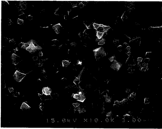
Figure 7. SEM photograph for cobalt oxide at the mixer temperature of 415 °C (reaction temperature and pressure: 430 °C and 340 bar).
