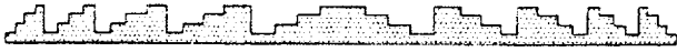
FIG. 3. Schematic diagram of multilevel K.E. surface profile as approximation of continuous shape, the surface profiles are quantized to have N number of levels (In this diagram, N is 4).
