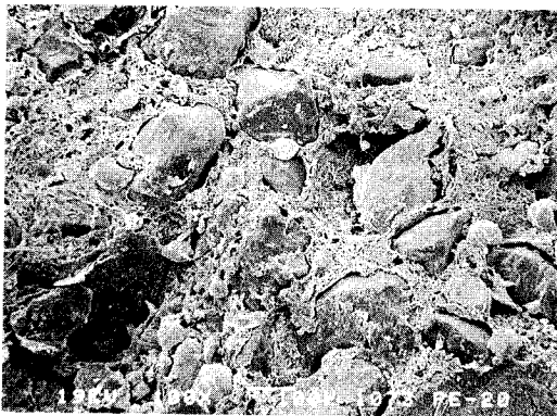
(c) PAE polymer-cement ratio, 20%
