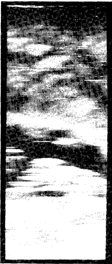
Figure 7. Raw SAR signal image acquired over Ottawa airport, Canada, using CCRS's C-band SAR system. Flight direction is from top left to top right in the image.
