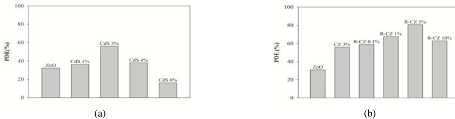
Fig. 1. Photocatalytic decomposition efficiency of O-xylene (PDE, %) of (a) ZnO particle and CdS/ZnO and (b) RGO/CdS/ZnO Photocatalyst.
