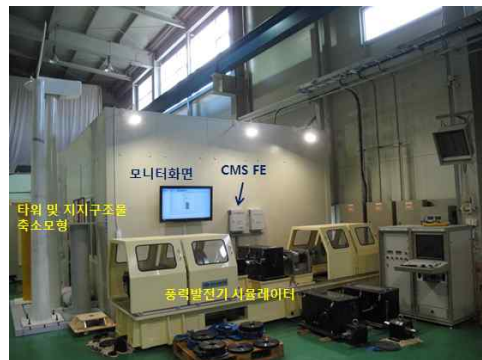
Fig. 1 Condition Monitoring System installed on Wind Turbine Simulator
