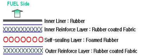
[Fig. 3] Material Property of Fuel Tank
