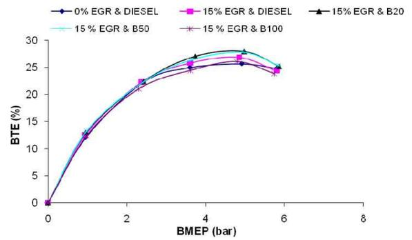
[Fig. 3] Variation of BTE Vs BMEP for different fuels with 15% EGR rate.
