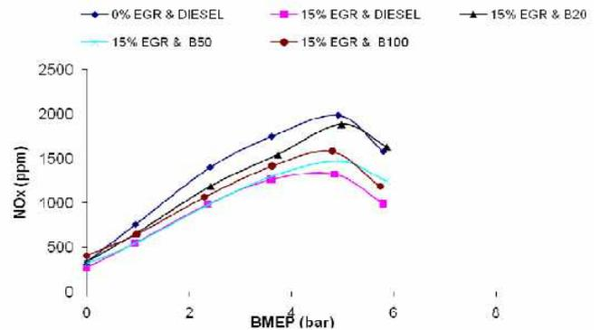
[Fig. 5] Variation of NOx Vs BMEP for different fuels with 15% EGR rate
