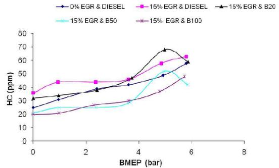
[Fig. 7] Variation of HC Vs BMEP for different fuels at 15% EGR rate.
