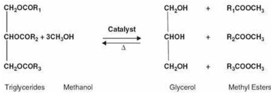
[Fig. 1] Typical transesterification reaction.
