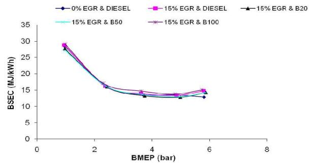
[Fig. 4] Variation of BSEC Vs BMEP for different fuels with 15% EGR rate.
