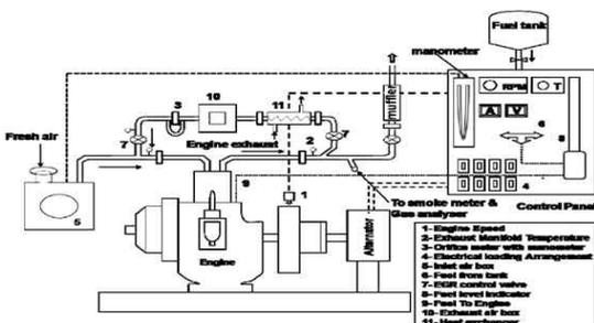
[Fig. 2] Schematic Line Diagram of Test Rig
