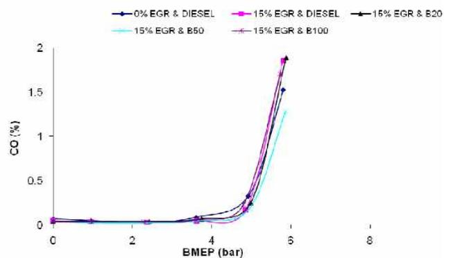
[Fig. 6] Variation of CO Vs BMEP for different fuels at 15% EGR rate
